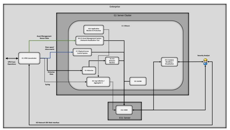
Figure 5.3 Monitoring/Data Collection Management Architecture Depicted using Generic Component Names
