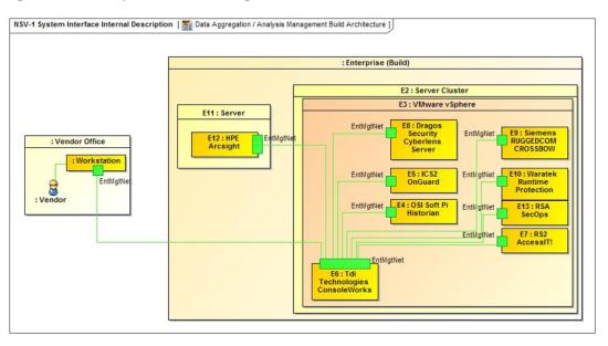
Figure 4.8 Enterprise Remote Management Lab Build Architecture
